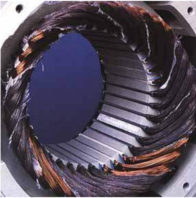
#1 Winding Single Phased (Y Connected)
