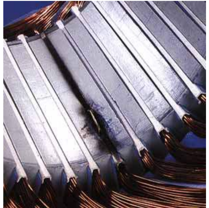
#6 Winding Grounded In Slot
