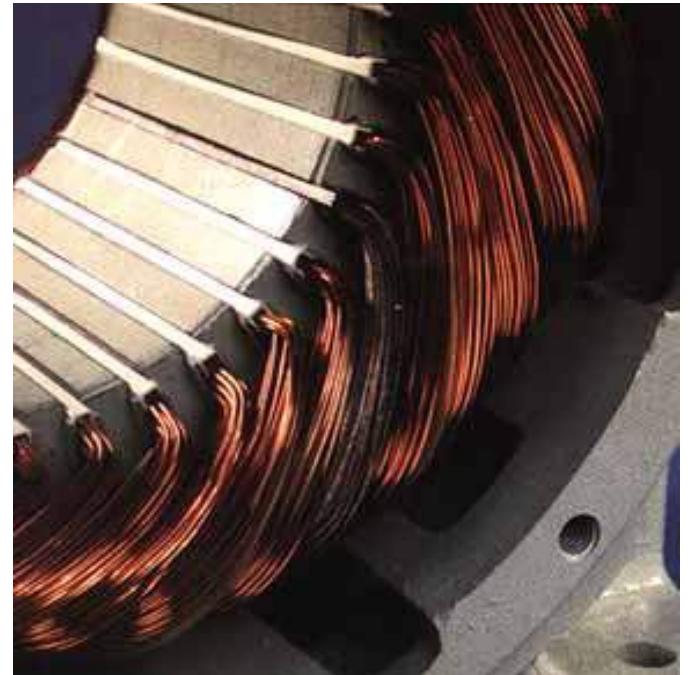
#8 Winding With Shorted Coil
