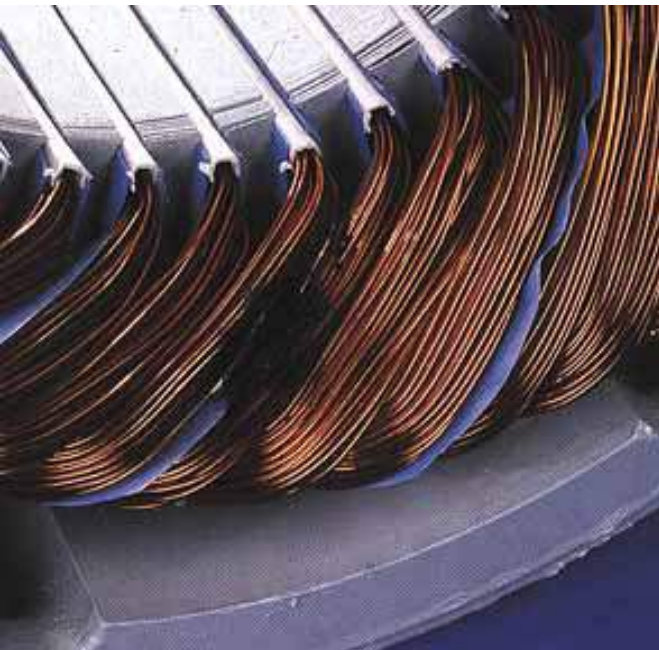
#3 Winding Shorted Phase to Phase
