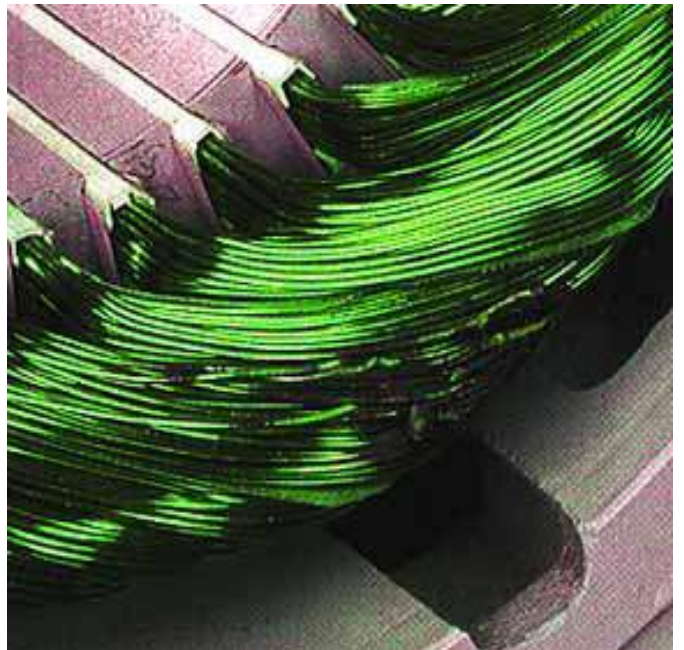
#4 Winding Shorted Turn To Turn
