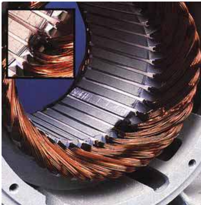
#7 Winding Grounded At Edge Of Slot
