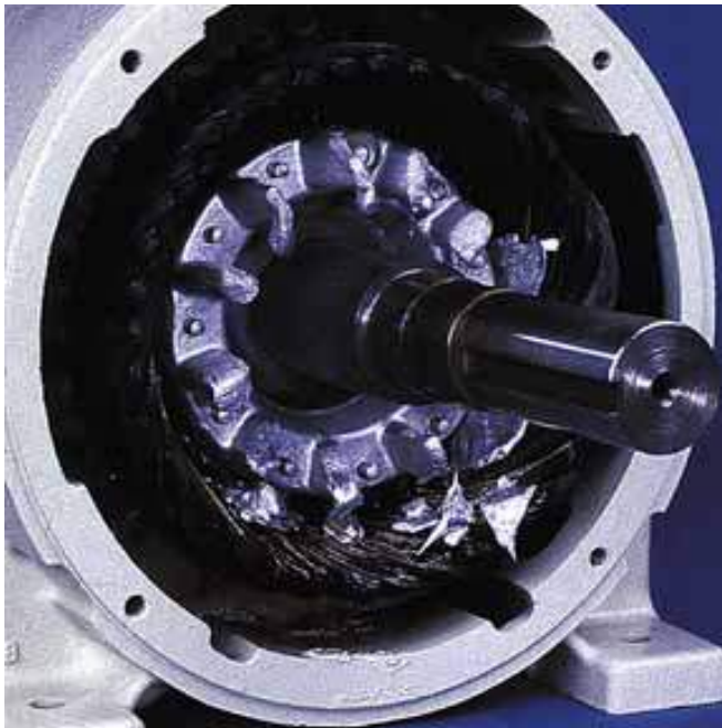
#11 Damage Caused By Locked Rotor
