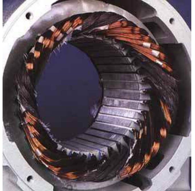
#2 Winding Single Phased (Delta Connection)
