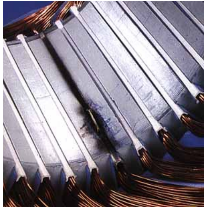
#6 Winding Grounded In Slot
