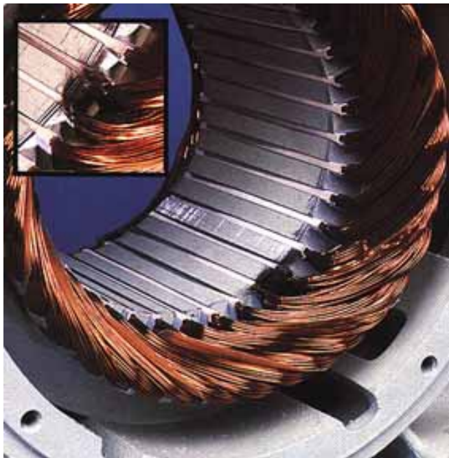
#7 Winding Grounded At Edge Of Slot
