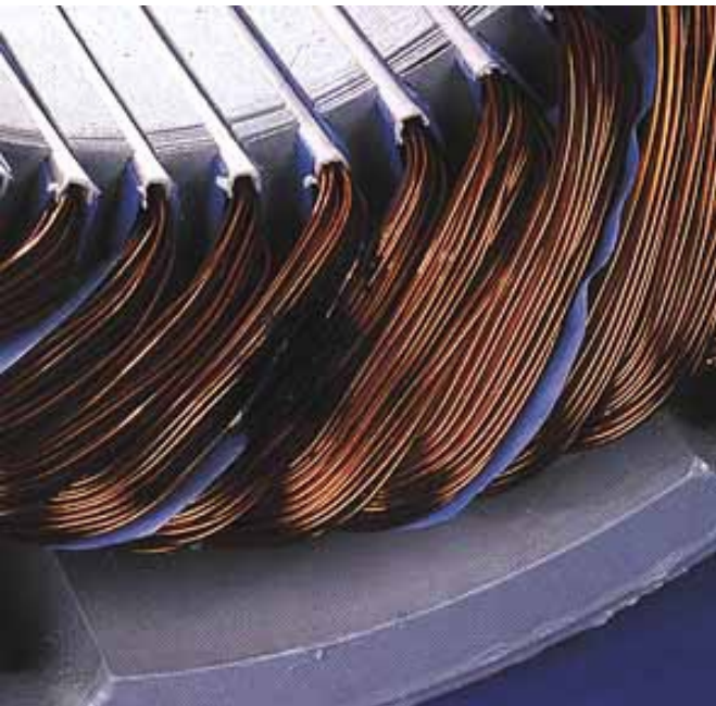
#3 Winding Shorted Phase to Phase
