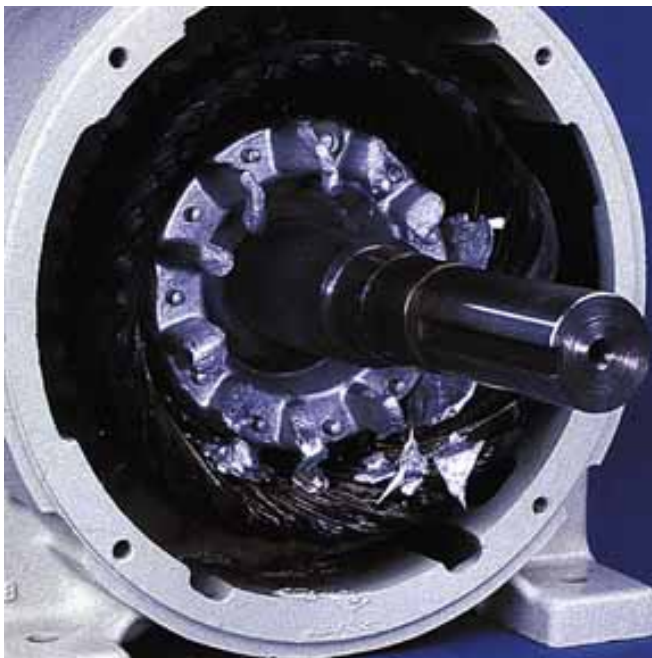
#11 Damage Caused By Locked Rotor
