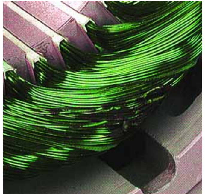
#4 Winding Shorted Turn To Turn
