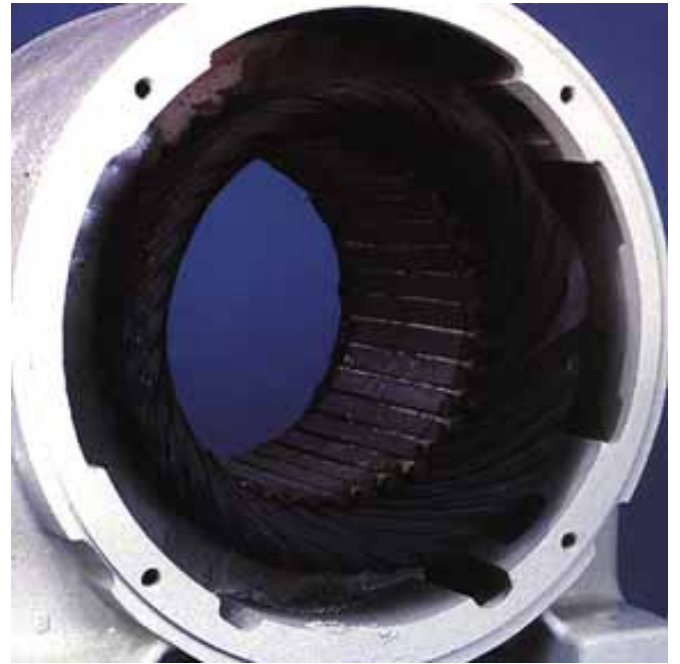
#10 Damage Due To Overload
